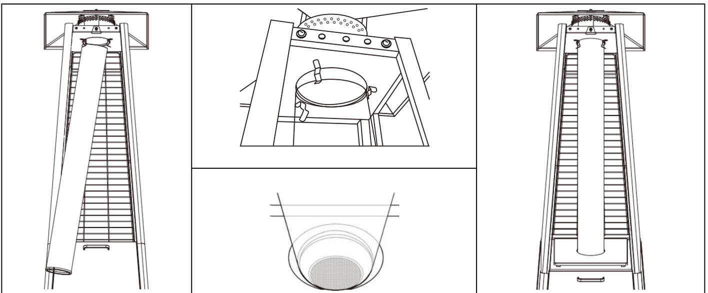
**STEP 9:** Fix Rubber Ring (6) into the bottom of Glass Tube (5). Insert the top end of glass tube into the bottom hole of Flame Screen (2) as much as possible. Keep glass tube vertically and sit it in the hole of Plate Cover (8).
