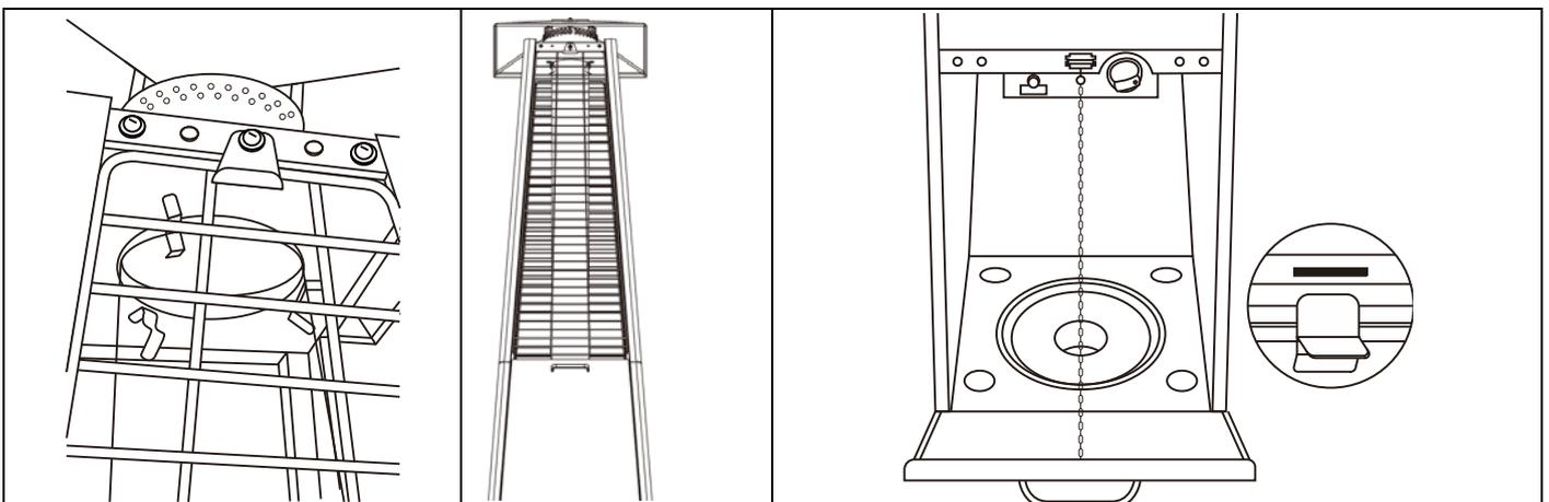
**STEP 10:** Assemble Mesh Guard (4) in the front. Loose 4pcs screws to keep 4pcs Guard Fastening Plates down and firmly in place.
