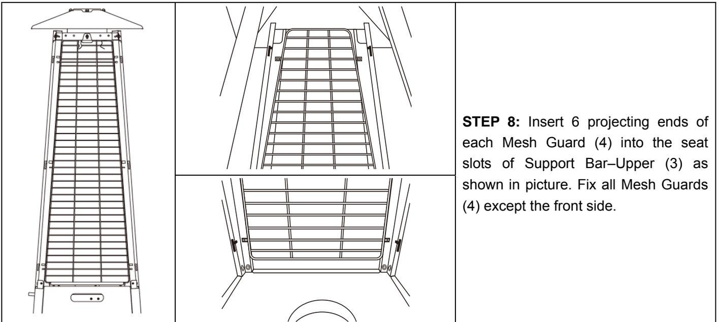
**STEP 8:** Insert 6 projecting ends of each Mesh Guard (4) into the seat slots of Support Bar–Upper (3) as shown in picture. Fix all Mesh Guards (4) except the front side.
